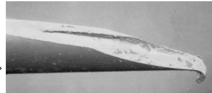
Reused needle at x370 magnification
