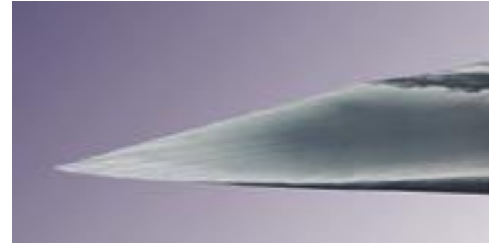
New needle at x370 magnification
