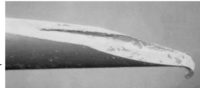
Reused needle at x370 magnification
